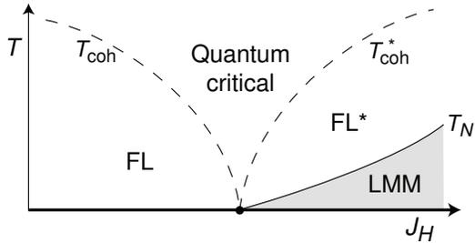
Fig. 5. Phase diagram near the conjectured FL to LMM quantum transition. The two distinct energy scales are manifested by the differing exponents by which  $T_N$  and  $T_{\text{coh}}$  (or  $T_{\text{coh}}^*$ ) approach the quantum critical point.
