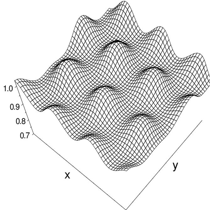
*Figure 4.* Spatial form of  $\langle \varphi_\mu(\mathbf{r}) \rangle$  in the SC+SDW phase. Notice the vertical scale, which shows that the overall modulation in the size of the order parameter is quite small. The numerical results were obtained by Ying Zhang and reported in [9].
