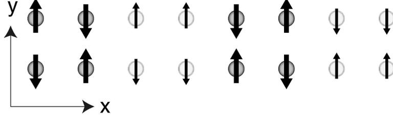
Figure 1. A bond-centered, collinear SDW at the wavevector  $(3\pi/4, \pi)$ . The size of the arrow represents the mean spin moment, while the shading of the circle is the electron density. The sliding degree of freedom corresponds to a shift in the position of the light and dark circles.
