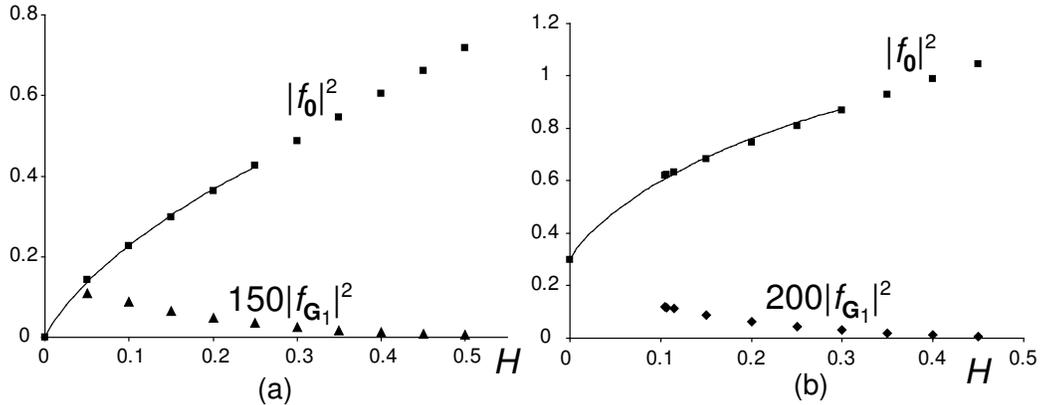
*Figure 5.* Magnitudes of the elastic scattering peaks in (15) obtained by the spatial Fourier transform of results like those in Fig 4. The field  $H$  is measured in units of  $H_{c2}^0$ , the value of the critical field at which all four phases meet in Fig 2. The plot (a) is at  $s = s_c$ , while (b) is for  $s < s_c$ . All other couplings are identical to those in Figs 3 and 4. The numerical results were obtained by Ying Zhang and reported in [9].
