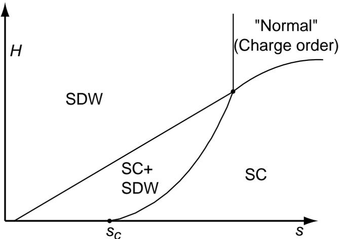
Figure 2. Zero temperature phase diagram of the model  $\mathcal{Z}$  defined in (8) and (9); from Refs. [5] and [9]. The phases have the following expectation values: (i) SC:  $\langle \varphi_\mu \rangle = 0$ ,  $\langle \psi \rangle \neq 0$ , (ii) SC+SDW:  $\langle \varphi_\mu \rangle \neq 0$ ,  $\langle \psi \rangle \neq 0$ , (iii) SDW:  $\langle \varphi_\mu \rangle \neq 0$ ,  $\langle \psi \rangle = 0$ , and (iv) "Normal":  $\langle \varphi_\mu \rangle = 0$ ,  $\langle \psi \rangle = 0$ .
