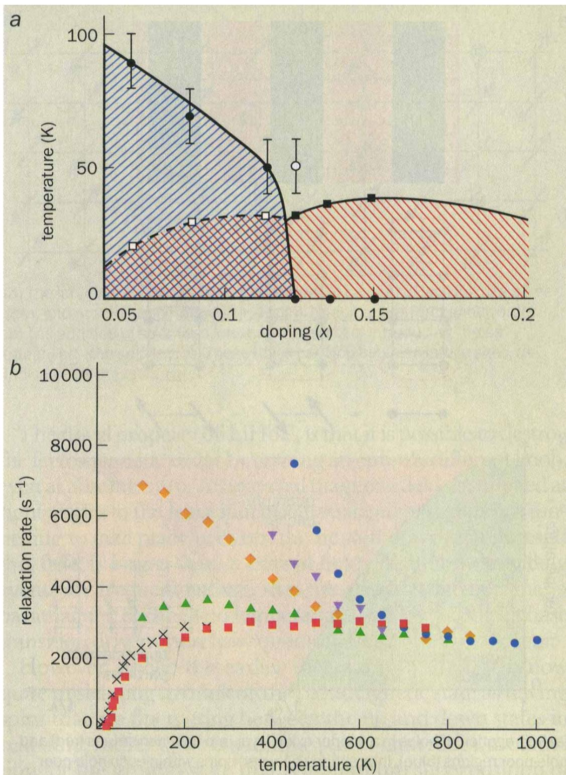
(a) Phase diagram of  $\text{La}_{2-x}\text{Sr}_x\text{CuO}_4$  as measured by the magnetic resonance experiments at MIT (Hunt *et al* [4]). There is quasi-static charge stripe order, over the blue hatched region. Superconductivity is present in the red hatched regions. The measurements indicate quasi-classical wave (particle) behavior at low (high) doping.
