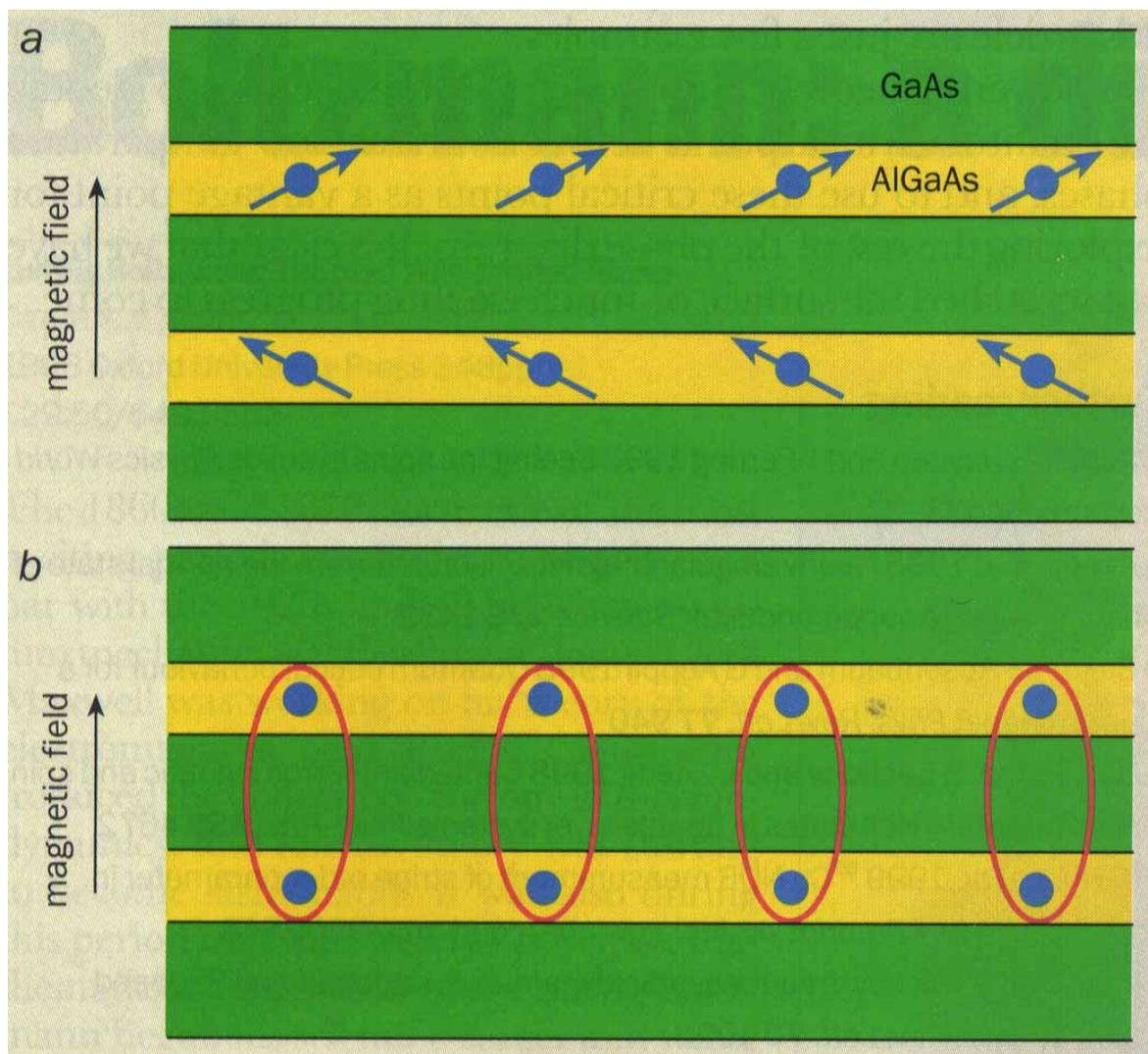
Electrons are confined within two two-dimensional quantum wells in a structure consisting of alternating layers of gallium arsenide (green) and aluminium gallium arsenide (yellow) [10]. The two possible magnetic phases shown have been observed in recent experiments. These phases are separated by a quantum phase transition. The phase diagram can be explored by varying the spacing between the layers, the direction of the magnetic field (not shown) through the sample and various other parameters.
